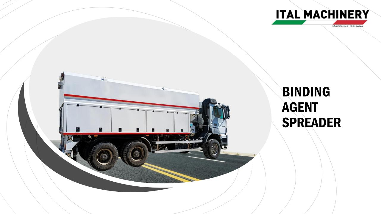
Binding Agent Spreader is a well-designed and reliable machine that you need for surface stabilization. Thanks to its automatic control system, this mobile spreader ensures that the filler, cement, lime etc. like powder materials spread on the surfaces at desired ratios. Its functional design guarantees the best spreading performance as well as easy usage.
